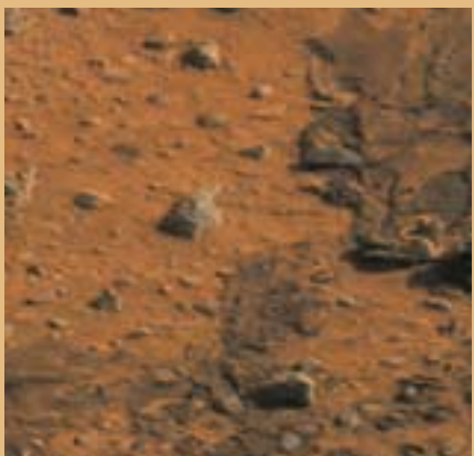
DRAG MARKS, left by the air bags as they were retracted, indicate a cohesive soil—perhaps electrostatically charged dust or a weakly cemented “duricrust” like that seen by Viking.
